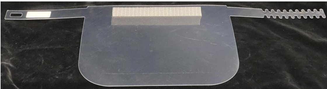
Face shield as received (with a protective plastic sheet on one side of the ocular)
